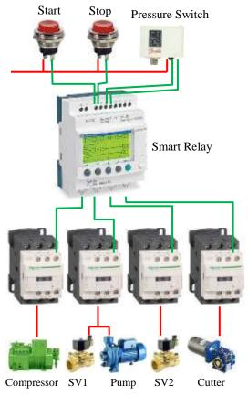
Figure 4. Single Line Diagram
