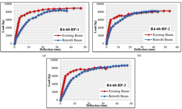
(c) Fig. 6. Curve of the relationship between the load and deflection of retrofit beams with initial loading reaching the peak load: (a) R4-60-BP-1, (b) R4-60-BP-2 and (c) R4-60- BP-3
