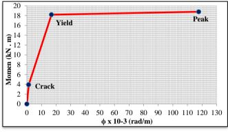
Fig. 3. The moment-curvature relationship of reinforced concrete beam specimen for determining the initial loading
