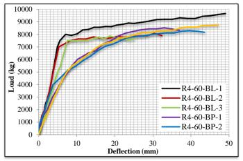
Fig. 7. Combined load and deflection curve of retrofit beams with initial damage variations
