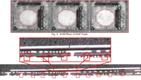
Fig. 5. DAF Voids in Cross Section Analysis
