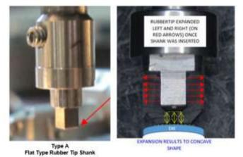
Fig. 3. Flat Type Rubber Tip Shank
