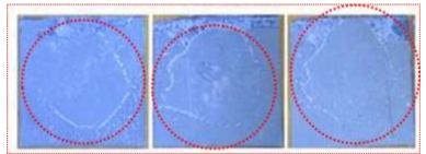
Fig. 6. Optical Photo of DAF Voids
