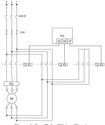
Figure 6. Star-Delta Wiring Circuit.
