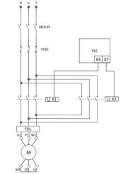
Figure 4. Forward-Reverse Wiring Circuit
