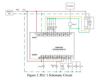
The output components used in this system are indicator lamp, buzzer, and magnetic contactors. Magnetic contactors are used to regulate the work of 3 phase motor.
