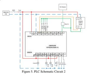
The output components of PLC 2 are indicator lamp, buzzer and magnetic contactors. Wiring circuit for magnetic contactors can be seen in Figure 6. There are three magnetic contactors are used, namely main contactor, star contactor, and delta contactor.
