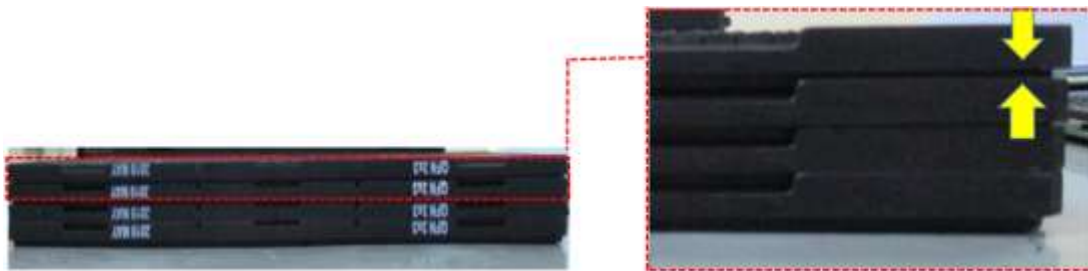
Fig. 4.0 Actual filed up trays with dislodged units inside.
