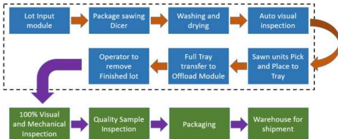
Fig. 1.0 Process flow of a Standalone package sawing machine with auto-pick and place
