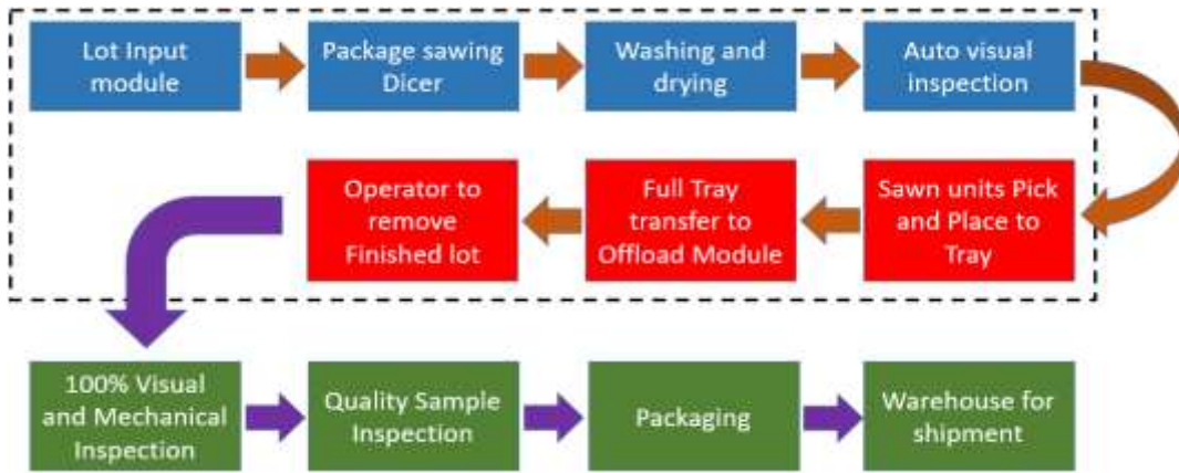
Fig. 2.0 Process flow where the package chips out happened.
