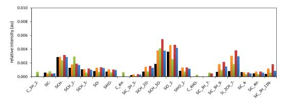
Fig. 3. TOF-SIMS negative scan molecular fragments from the polyamide surface at different process conditions.
