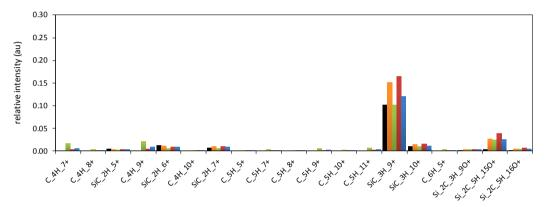
Fig. 2. TOF-SIMS positive scan molecular fragments from the polyamide surface at different process conditions.
