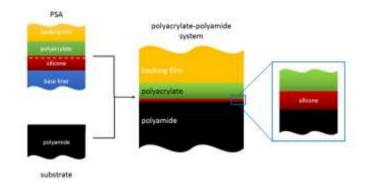
Fig. 1. Build-up of the adhesion interface, from polyacrylate-based PSA and polyamide substrate, with residual silicone [6].
