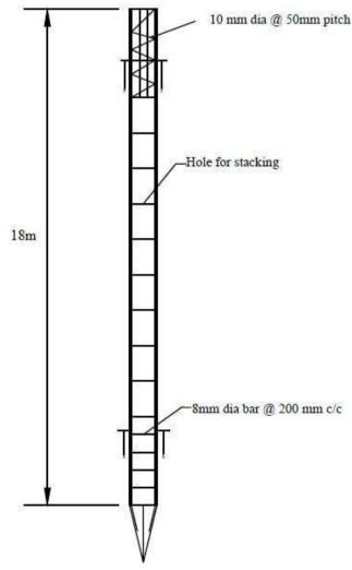
Fig. 5. Pile Reinforcement
