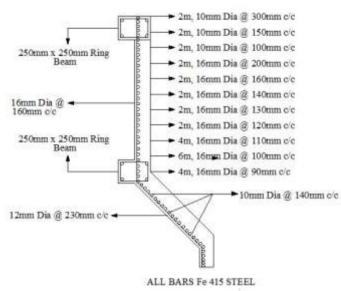
Fig. 3. Silo Reinforcement Details.
