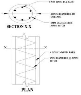
Fig. 4. Column Reinforcement Details
