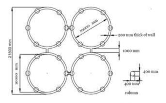
ALL DIMENSION IN ARE MM Fig. 1. Silo Plan.
