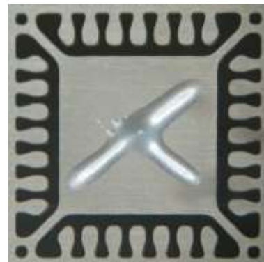
Fig. 3. Inconsistent Dispense Pattern
