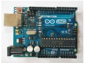
Fig. 3. Arduino Uno board
