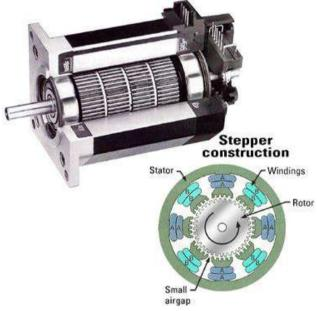
Fig. 1. Stepper Construction
