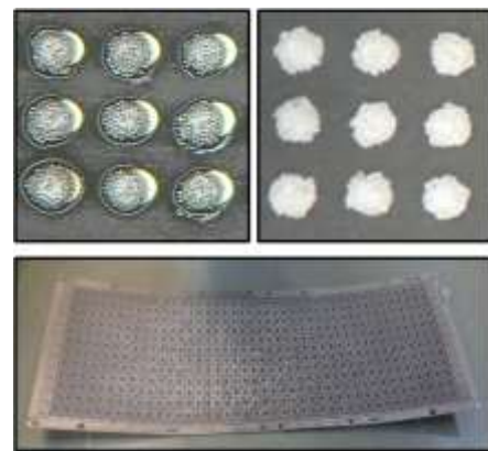
Fig. 2. Package defect manifestation.
