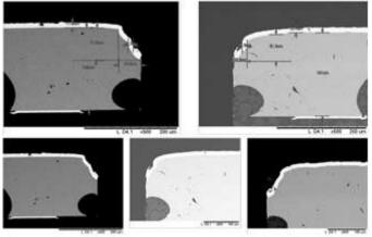
Fig. 5. Cross-sectional images of leads after the treatments and tin plating.
