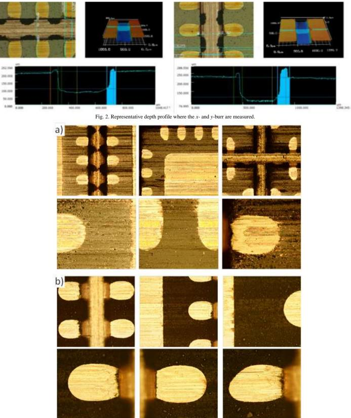
Fig. 3. Representative images of Cu terminations a) after buffing and b) after chemical deflash and water jet process.
