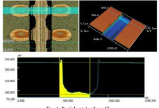
Fig. 1. Partial-cut depth profile.
