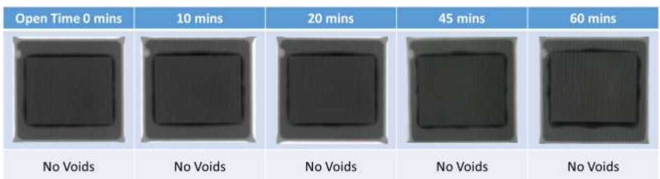
Fig. 7. Epoxy Voids Verification
