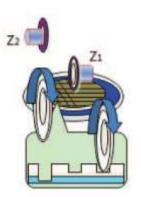
Fig. 1. Wafer Sawing Process with Step Cut [2]
