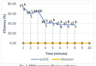
Fig. 7. HHO generator efficiency with time
