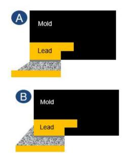
Fig 2. (A) Conventional QFN, (B) Automotive requirement with visually detectable solder joint through wettable flank.
