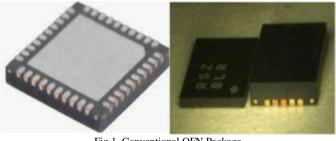
Fig 1. Conventional QFN Package
