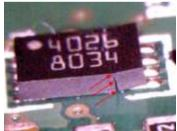
Fig. 2. DFN package crack.
