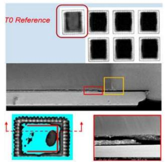
Fig. 1. Delamination in a leadframe-based device.
