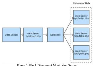
Figure 2. Block Diagram of Monitoring System
