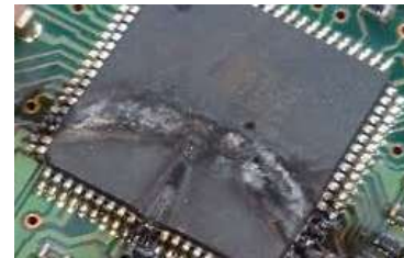
Fig. 2. Example of ESD/EOS-damaged QFP device.
