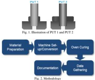
PUT (pick-up tool) 1 is the existing design of the indirect material currently used on die attach process while the PUT 2 is modified with larger backside support.
