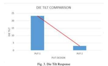
Comparison of the result for both PUT design shows improvement in the die tilt response which the second design of PUT is observed to have lower tilt. A PUT with enough support tends to improve the tilting behavior of the silicon die during the bonding process yet the existing material partnered with larger tool produces more variation during the process.
