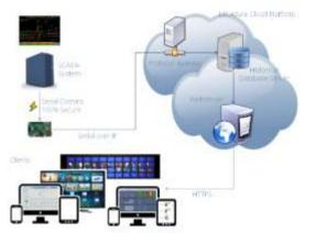
Fig. 5: Cloud computing application in substation automation system
