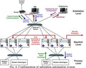
Fig. 4: Configuration of substation automation system
