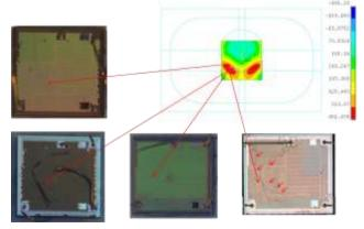
Fig. 4. Stress analysis result showing location of maximum die stress and mapping with actual die crack.
