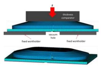
Fig. 3. Package finite element model.
