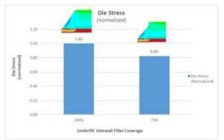
Fig. 4. Die stress vs underfill sidewall coverage (%).
