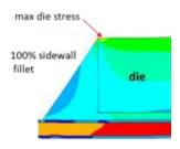
Fig. 3. Stress analysis result showing location of maximum die stress.
