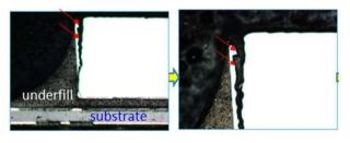
Fig. 2. Die crack at the side of the silicon die.
