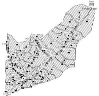
Figure 2. The Display of Linei River Catchment Area Existing SWMM Model
