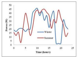
Fig. 4. The power generated by wind turbine in winter and summer
