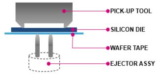
Fig. 3. Illustration of the location of vacuum hole and ejector needle for PUT#1.
