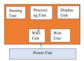
Fig. 1. The Block Diagram of Smart Waste-bin monitoring system
