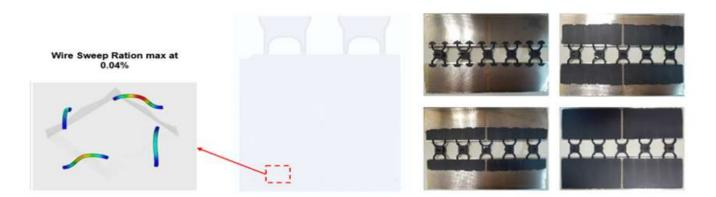
Fig. 2. Mold flow simulation with highlighted point at the critical area near the air vent side. Short shot reveals a balanced mold compound flow.
