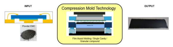
Fig. 1. Compression molding process using granular molding compound on a single cavity with film assist molding.
