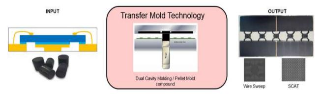
Fig. 3. Transfer molding process using pelletized molding compound on a dual cavity.
