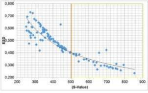
Fig. 3. Graph of the relationship between entrance surface dose (ESD), exposure Index. (S-Value) and guidelines radiation dose BAPETEN
