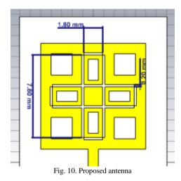
Fig. 10 and Fig. 11 shows the proposed antenna design and its return loss characteristics respectively.
