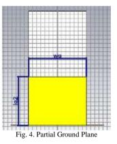
With the introduction of partial ground plane the bandwidth has considerably increased to 4.21GHz (from 2.77GHz to 6.98GHz) and the antenna resonates at 3.4 GHz and 5.8GHz as shown in Fig. 5.
