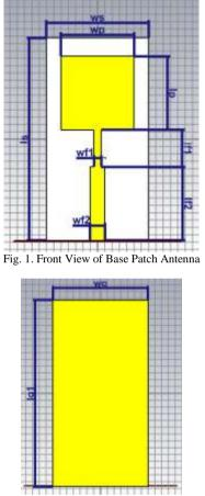
Fig. 2. Back View of Base Patch Antenna
