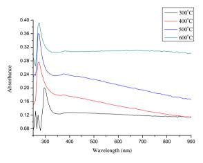
Fig. 5. The absorption graph of ZnO thin films (a) at 300  $^{\circ}\rm C$  (b) at 400  $^{\circ}\rm C$  (c) at 500  $^{\circ}\rm C$  and (d) at 600  $^{\circ}\rm C$
