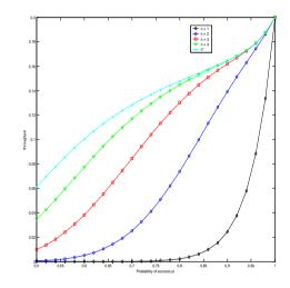
Figure 3: Throughput vs. probability of success Pi for the stop-and wait M\_0  $$\operatorname{protocol}$$
