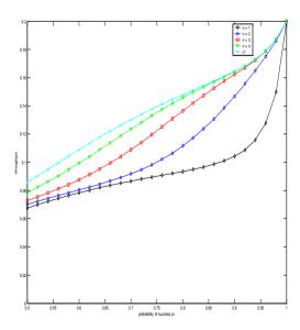
Figure 4: Throughput vs. probability of success Pi for the stop and wait M\_1 protocol
