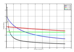
Figure 6: Throughput vs. number of receivers K for the Go-back-N M\_1 protocol
