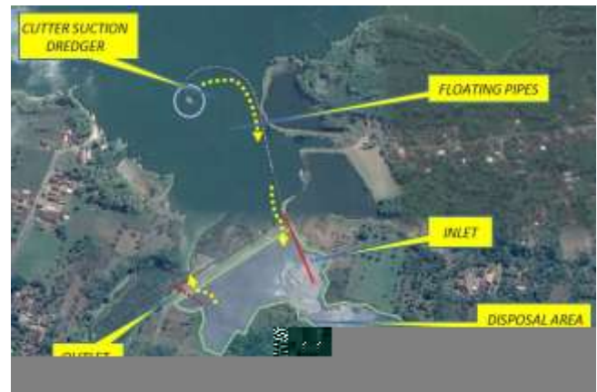
Fig. 4. Scheme of Sutami Reservoir Dredging Work
