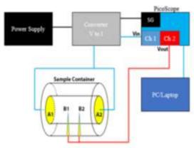
Fig. 1. Measurement system design.
