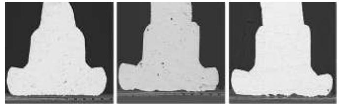
Fig. 2. Uneven wirebond ball height.
