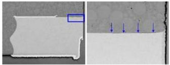
Fig. 1. Delamination along the EMC-to-carrier interface.
