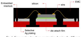
Fig. 6. Cross-sectional package construction showing the different components of the assembly.
