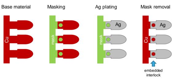
Fig. 4. Embedded interlock process flow.
