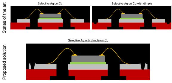
Fig. 5. Package cross-sectional construction using selective Ag on Cu, Selective Ag on Cu with dimple and the selective Ag with dimple on Cu.
