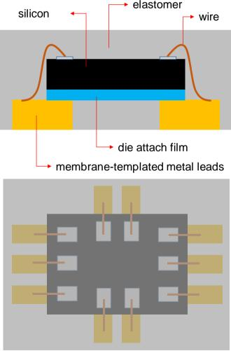
Fig. 3. Package cross-sectional (top) and top (bottom) views.
