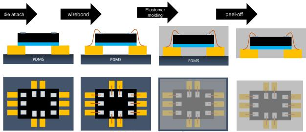
Fig. 2. Package assembly process flow.
