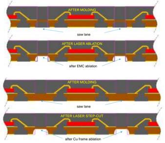
Fig. 3. Laser ablation of EMC (top) and Cu frame (below) to achieve step-cut QFN configuration.
