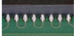
Fig. 1. Soldering miniscus of standard QFN (top) and QFN with wettable flanks (middle). Board mounted QFN with wettable flanks (bottom).
