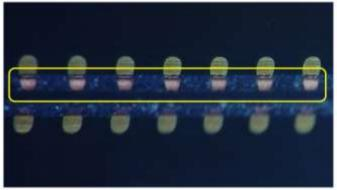
Fig. 4. Laser ablation of EMC resulting in step-cut configuration.
