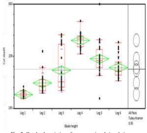
Fig. 2. Cut depth variation after conventional singulation.
