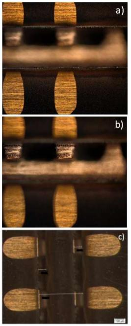
Fig. 5. Laser ablation of Cu frame with a-b) wide trench and c) two parallel narrow trenches resulting in step-cut configuration. b) Tilted view showing sidewalls with no heat affected zone (HAZ).
