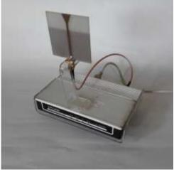
Fig. 21. Antenna connected to Wi-Fi Router
