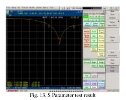
From the curve view on the Anlyzer network above (Figure 13), it appears that the working frequency channel slightly complains the small shift to 2,402 GHz which is still within the working range of the desired specification and does not differ much from the software simulation results (Figure 4). After doing the test of the S Parameter then next proceed to test the SWR value.
