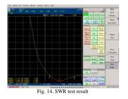
From the Figure 14, SWR test results can be seen at the position of working frequency 2.4 GHz then the value of SWR generated by the antenna is 1.045 which means that the antenna made already meets the standard criteria for SWR is  $\geq$ 2 and not much different from the software simulation results (Figure 6) which shows the position of SWR at the number 1.079. The last test was performed to test the value of the antenna impedance as follows.
