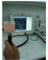
Fig. 12. Antenna test with network analyzer tool
