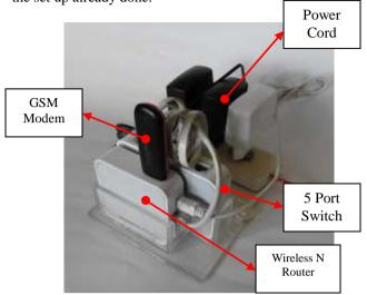
Fig. 22. GSM to internet protocol converter
