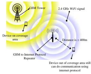
Fig. 20. Schematic of blank-spot area
