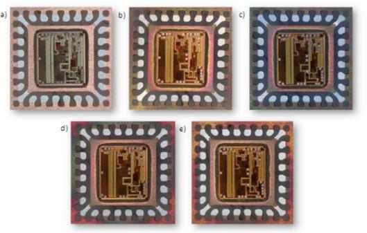
Fig. 1. Optical images of samples at a) time zero, b) after 24 h at 175 °C, and after exposure to c) water, d) 10 ppm Cl<sup>-</sup>, and e) 100 ppm Cl<sup>-</sup> solution followed by thermal treatment for 24 h at 175 °C.
