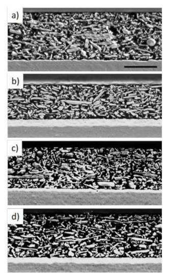
Fig. 6. SEM micrographs of samples pre-baked for 24 h at 175 °C followed by another 24 h at 175 °C. Prebaked samples are subjected to a) no treatment, b) water, c) 10 ppm Cl<sup>-</sup>, and d) 100 ppm Cl<sup>-</sup> solution before the second bake step.
