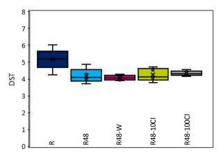
Fig. 4. DST results for samples pre-baked for 24 h at 175 °C followed by another 24 h at 175 °C. Prebaked samples are subjected to no treatment (R48), water (R48-W), 10 ppm Cl<sup>-</sup> (R48-10Cl), and 100 ppm Cl<sup>-</sup> (R48-100Cl) solution before the second bake step.
