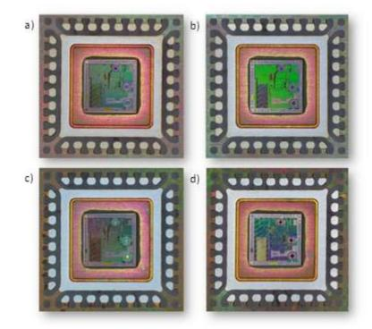
Fig. 2. Optical images of samples pre-baked for 24 h at 175 °C followed by another 24 h at 175 °C. Prebaked samples are subjected to a) no treatment, b) water, c) 10 ppm Cl<sup>-</sup>, and d) 100 ppm Cl<sup>-</sup> solution before the second bake step.
