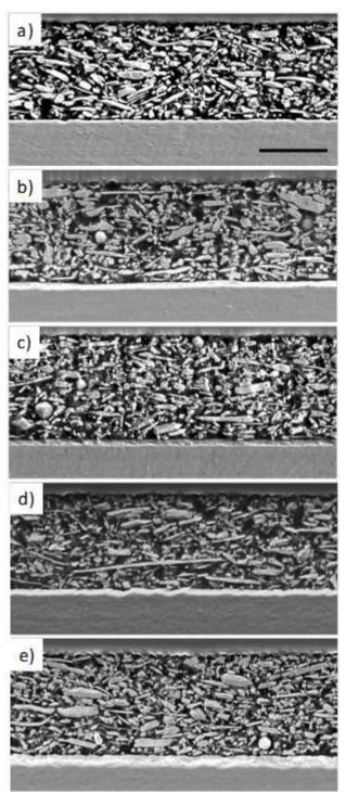
Fig. 5. SEM micrographs of samples at a) time zero, b) after 24 h at 175 °C, and after exposure to c) water, d) 10 ppm Cl<sup>-</sup>, and e) 100 ppm Cl<sup>-</sup> solution followed by thermal treatment for 24 h at 175 °C. Scale bar = 2  $\mu$ m.
