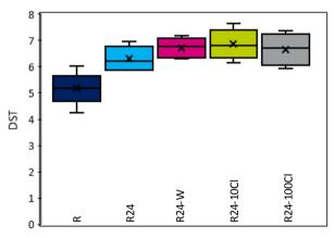
Fig. 3. DST results for samples at time zero (R), after 24 h at 175 °C (R24), and after surface treatment [water (R24-W); 10 ppm Cl<sup>−</sup> (R24-10Cl); and 100 ppm Cl<sup>−</sup> (R24-100Cl)] followed by thermal treatment at 24 h at 175 °C.
