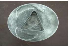
Fig. 2. Triangular Piston Crown
