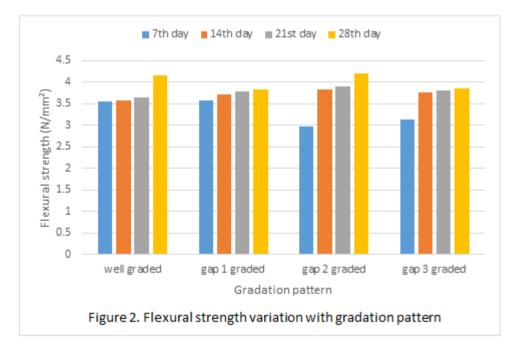
As observed from figure 2, the flexural strength of concrete was increased as the age increased for any particular gradation pattern. The flexural strength increased marginally during the early stages but increased abruptly at 28 days for the well graded aggregate concrete. For gap 1 to gap 3 aggregates, the concrete increased more at its early ages. On a close observation of figure 2, the early flexural strength for gap 1 (minus 5mm) aggregate is higher due to the presence of
