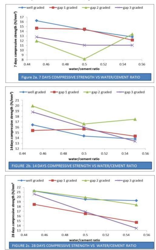
graded in that order for 14<sup>th</sup> day, 0.55 w/c ratio concrete (Figure 2b).
