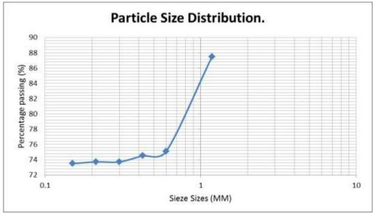
Fig. 1. Chart showing the relationship between percentage passing and sieve sizes.
