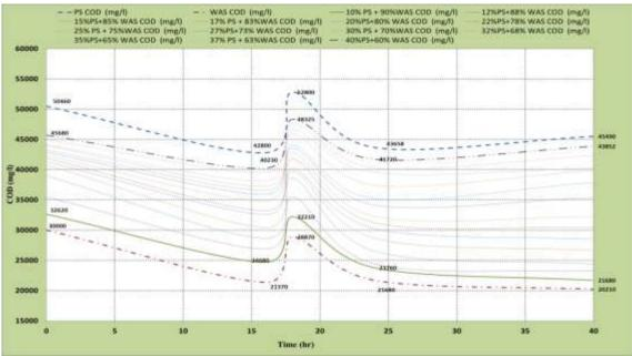
Figure (3) COD versus Time for Different Sludge Types from El Berkah WWTP.
