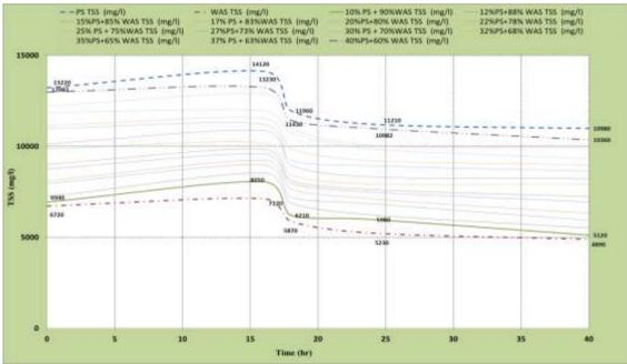
Figure (4) TSS versus Time for Different Sludge Types from El Berkah WWTP.
