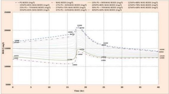
Figure (6) BOD<sub>5</sub> versus Time for Different Sludge Types from Zenein WWTP.
