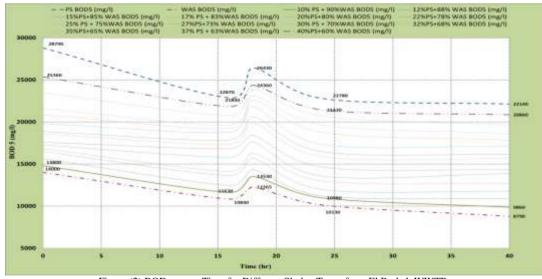
Figure (2) BOD<sub>5</sub> versus Time for Different Sludge Types from El Berkah WWTP.
