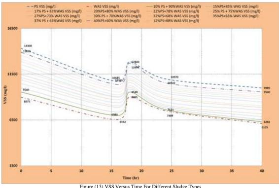
Figure (13) VSS Versus Time For Different Sludge Types From El-Gabal Al-Asfar (contract (16)) WWTP.
