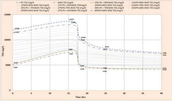
Figure (8) TSS versus Time for Different Sludge Types from Zenein WWTP.
