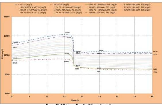
Figure (12) TSS Versus Time For Different Sludge Types From El-Gabal Al-Asfar (contract (16)) WWTP.
