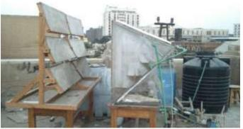
Fig. 2. The acrylic pilot plant [8]
