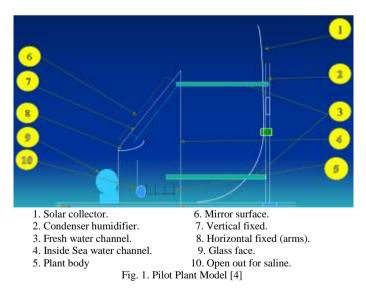
Meshaly, O. et al., [4] made a model for that unit figure (1) and proved that this idea is applicable to produce fixed quantity and good quality for produced desalinated water. His study covered the main elements affected the unit operation and obtains its best values for the system success. Also it
