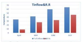
Fig. 6. Temperature of inflow raw water and the recovery ratio
