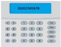
Fig. 3. Dialup or GSM sensor controller.
