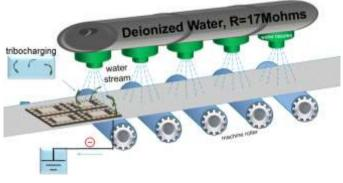
Fig. 1. Waterjet deflash process illustrating the tribocharging.
