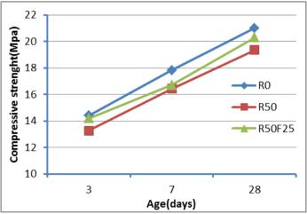
Fig. 5.1. Compressive strength with age for W/C of 0.3
