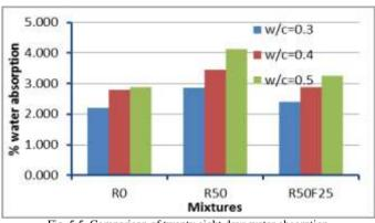
Fig. 5.5. Comparison of twenty eight days water absorption
