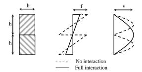
a. section b. bending stress c. shearing stress Fig. 2. Slip and partial interaction for two rectangular beams (Johnson, 1975).
