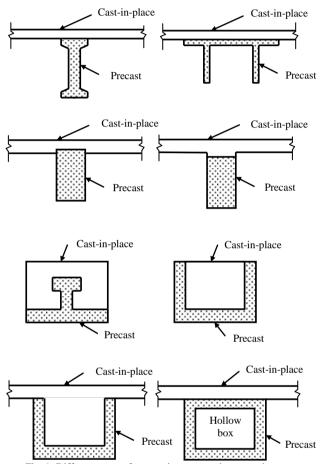
Fig. 1. Different types of composite concrete beam sections.
