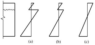
Fig. 3. Strain diagrams in (a) noncomposite, (b) partially composite, (c) full composite beam.
